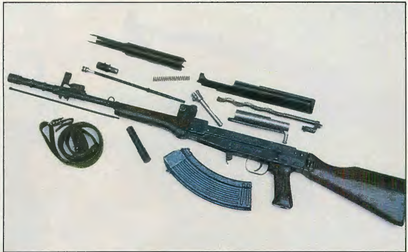
PRC Type 81 rifle, caliber 7.62x39mm, fieldstripped with sling and 30-round magazine.
